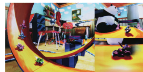
Figure 1: The extended 3D Mark Mobile OpenGL ES 1.X (left) and 2.0 (right) engines running on ASIC implementations of our architecture. Extensions include primitive processing and per-fragment shading presented in the paper with content featuring on-chip subdivision for the curtain, coal pot and bear, on-chip silhouette rendering-based soft shadow mapping and particle systems rendering with application-specified geometry shaders, Cook-Torrance shading on the main characters and other scene objects and Fresnel-like planar reflections on the floor.
