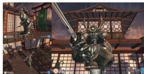
Figure 1: The extended 3D Mark Mobile OpenGL ES 1.X (left) and 2.0 (right) engines running on ASIC implementations of our architecture. Extensions include primitive processing and per-fragment shading presented in the paper with content featuring on-chip subdivision for the curtain, coal pot and bear, on-chip silhouette rendering-based soft shadow mapping and particle systems rendering with application-specified geometry shaders, Cook-Torrance shading on the main characters and other scene objects and Fresnel-like planar reflections on the floor.
